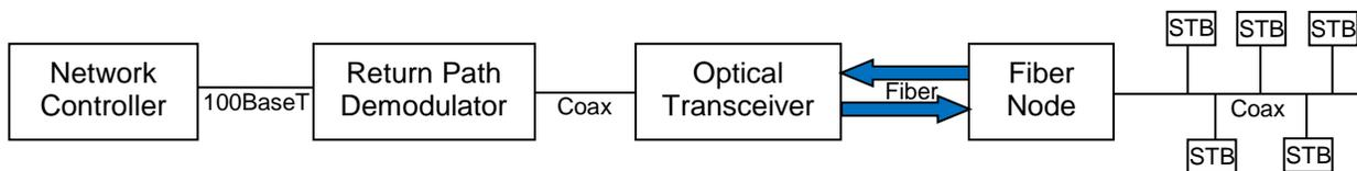
*Figure 1 MSO HFC Return Channel Topology*
